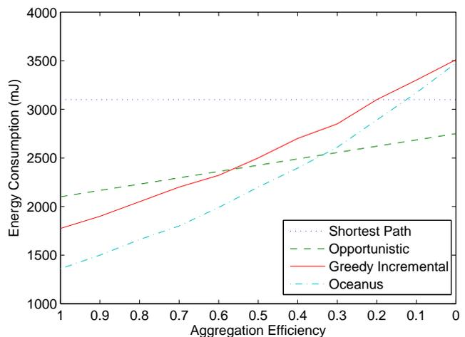
Fig. 8. Energy Consumption vs. Aggregation Efficiency, Network 3
