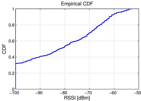
**Figure 4: Fraction of APs scanned at or below a signal strength on UIUC campus roads. A link can be established with as little as -90dBm.**
