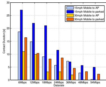
Figure 6: Link duration to an AP Vs a link between moving and parked vehicles.
